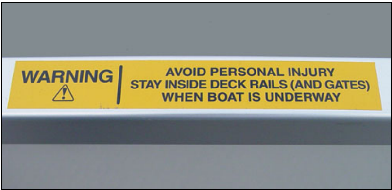
Figure 2-1 Safety Labels Located On Top Of Deck Rails
